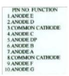
The pin connections for the seven-segment display are shown in the diagram above. It is a common-cathode display, which means that the negative side of the diode elements are connected together, and should be connected to ground. The positive side of each diode should be connected, through a 1 k $\Omega$  resistor, to the appropriate digital output of your Arduino board. Be sure to use a resistor: if 5 V is applied directly across a diode, it will be destroyed by the large current that flows.
